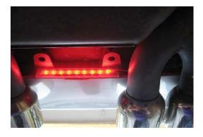
Peel adhesive backing and mount led plate on flat surface facing directly at exhaust plate. Route wiring behind other facia mounting tabs to keep away from exhaust.
