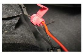
Connect red wire to brown wire and black to black. Make sure wires are seated correctly and close connector with pliers.
