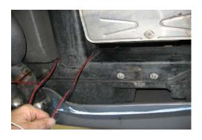
The goal is to route the wires toward the rear side marker light. I used a hangar to fish wires between rear compartment and frame rail in the corner. Bend the hangar so it will exit as shown. Tightly tape the wires to the end of the hangar and pull it through as shown. Patience may be required! This will keep the wire away from the exhaust.
