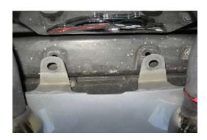
Directly behind the exhaust plate you will see these 2 rear facia mounting tabs. This is where the led plate will mount. Clean mounting area with alcohol.
