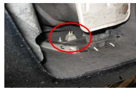
Next reach up inside the rear fender and locate the rear marker light. Twist 1/4 turn to the left and drop socket down so you can connect the led wires using supplied connectors.
